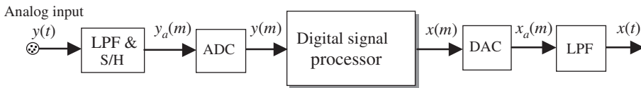
Figure 1.22 Configuration of a digital signal processing system with analogue input and output.
